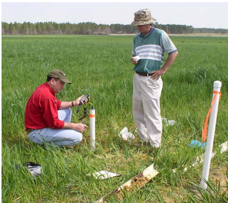
Steve Lawrence and Ken Monroe, USDA NRCS soil scientists, download data from a piezometer – data logger into a PDA (personal digital assistant). This data will be transferred to a computer database later.
